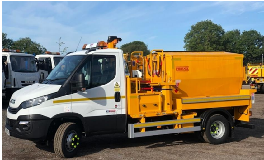
Hot-Box Pothole Repair Vehicle.
